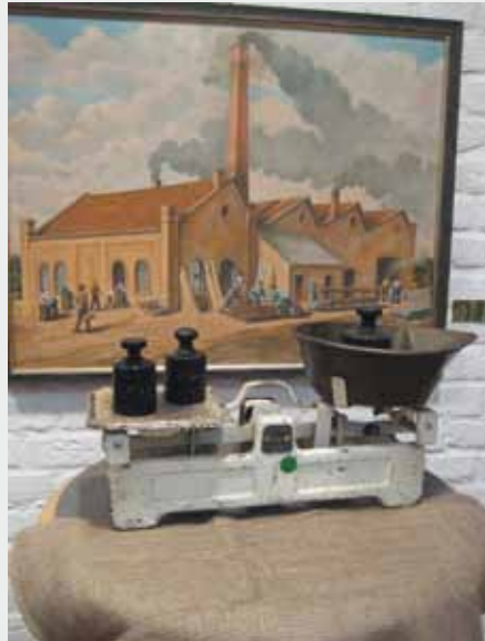
The platform scale works on the principle of the equal armed beam scale.
